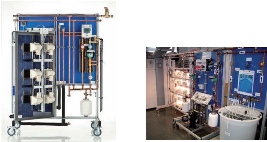
Figure 11: Mobile demo plant for a solar thermal flat collector (left), a hybrid collector containing solar thermal and heat pump systems (right), Source: Install+RES project
